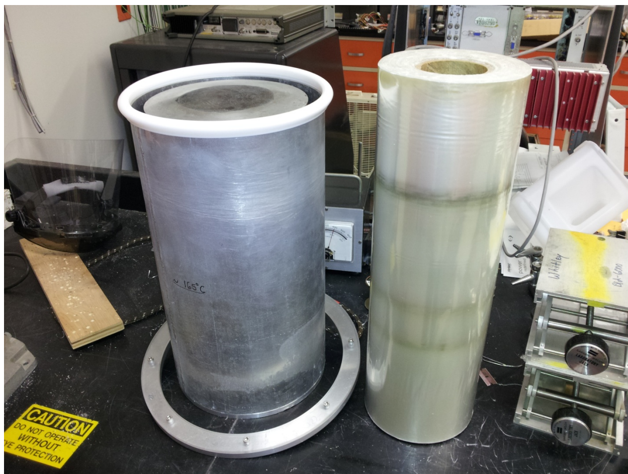
Figure 4.4: Polypropylene targets were made from an industrial roll of polypropylene manufactured by Exxon Chemicals. Material was heated and stretched before gluing to target frames.
