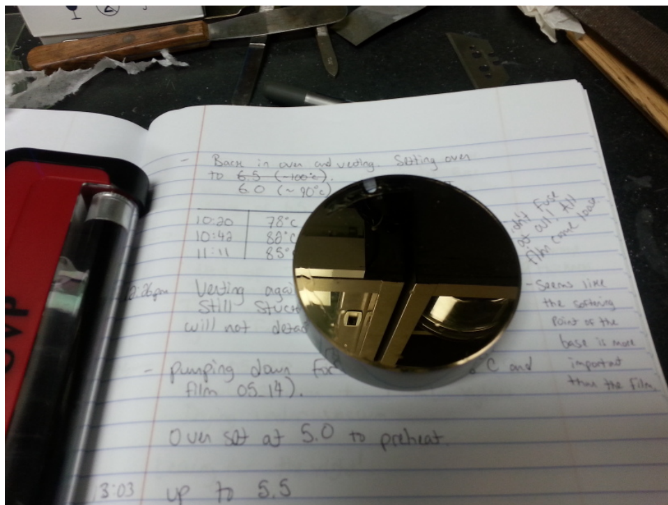
Figure 5.19: Plastic phoswich detector made by fusing a thin layer of plastic scintillator to a thick plastic scintillator disk in a vacuum oven. The top side of the thin layer is coated with a very thin layer of aluminium.
