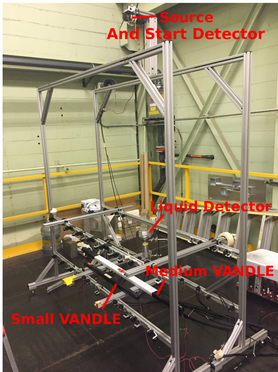
Figure 4.4: Neutron detector intrinsic detection efficiency measurement setup at Oak Ridge National Laboratory.
