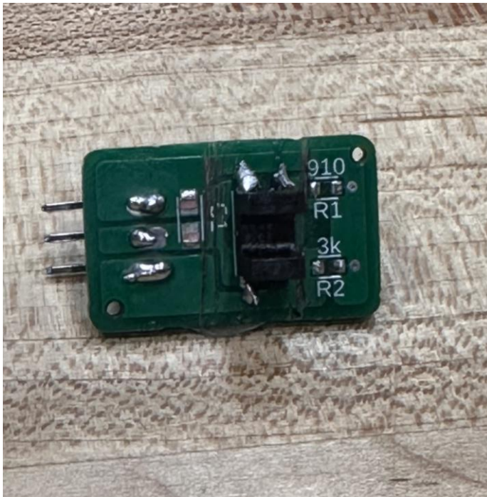
Figure 3.6 Circuit board layout for Rohm transducer
