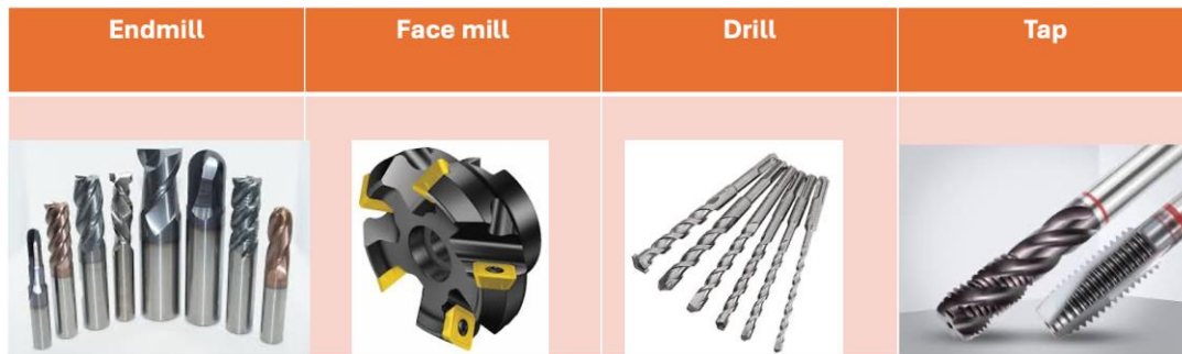
Figure 2.2 Visual representation of common milling tools.
