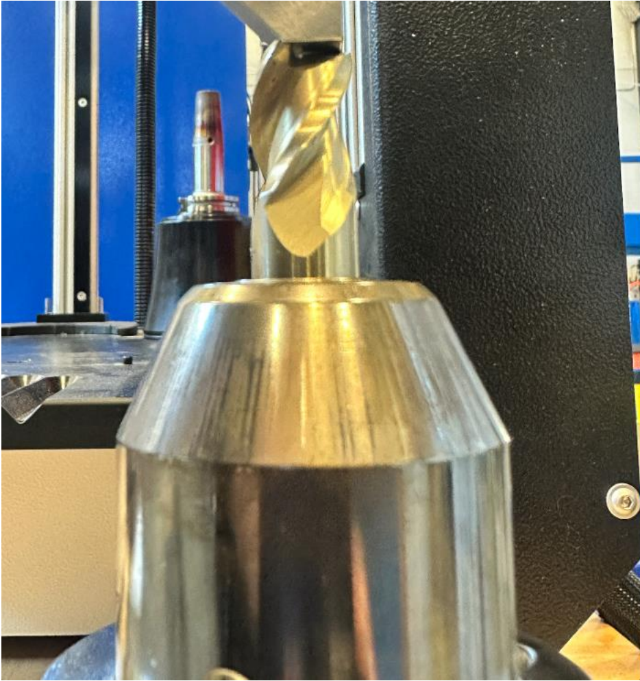
Figure 4.10 Tool setting for three-fluted endmill
