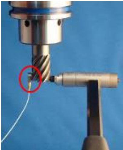
Figure 3.17 Modal tap testing accelerometer usage
