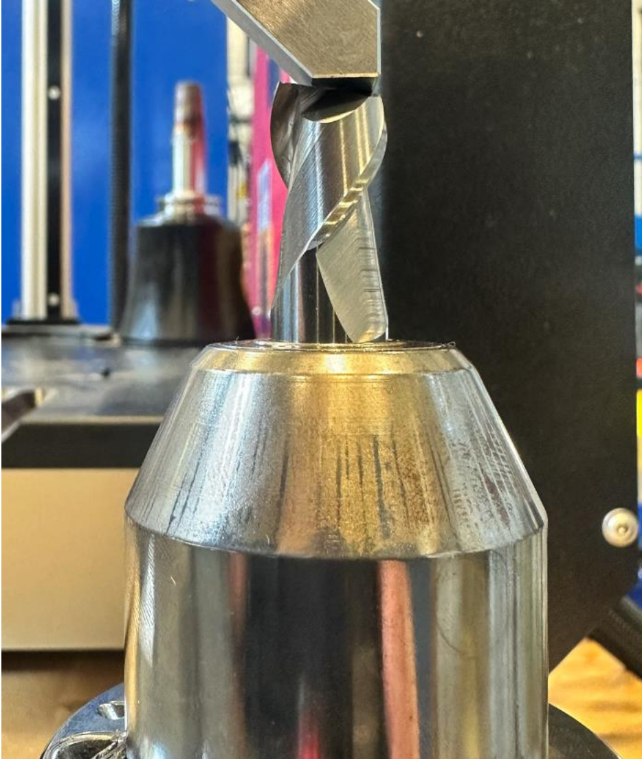
Figure 4.9 Tool setting for two-fluted endmill
