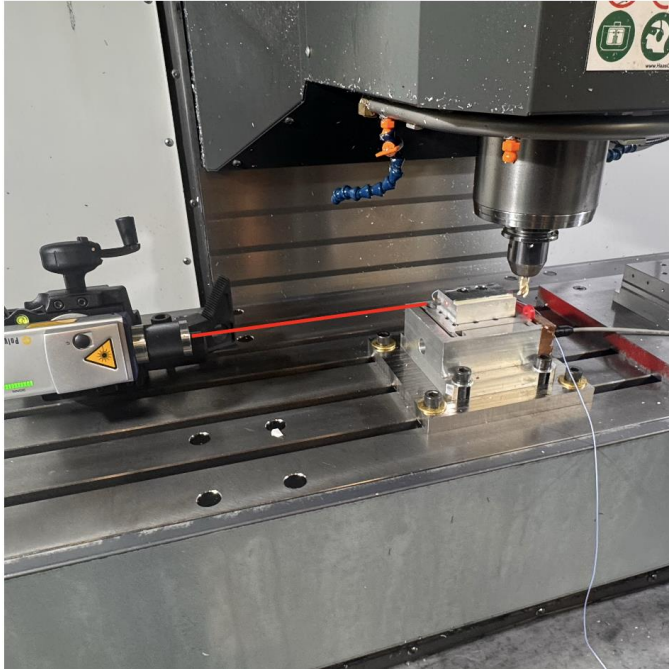
Figure 4.6 Laser vibrometer orientation mounted onto the worktable.
