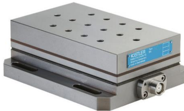
Figure 3.12 Kistler 9257 commercial grade force dynamometer.
