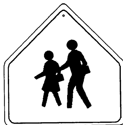
Advance School Crossing Sign (S1-1)
