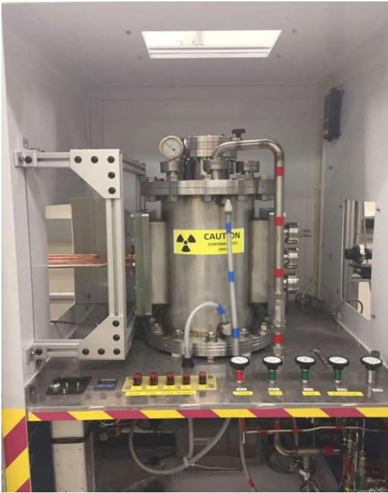
Figure 4.1 (Left) Compact Fuel Element Environmental Test (CFEET) Furnace and manual flow controls (Right) CFEET control panel and in-test monitoring of a sample during testing.
