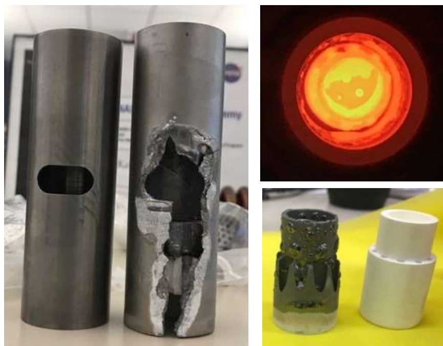
Figure D.7. (Right) Example of a W susceptor operated with an incompatible SiC sample holder. Direct contact of SiC and W resulted in low melting temperature compound formation and catastrophic failure of the susceptor. (Left) Example of incompatible BN stage operated with a W susceptor which resulted in the formation of undesirable boride phases.
