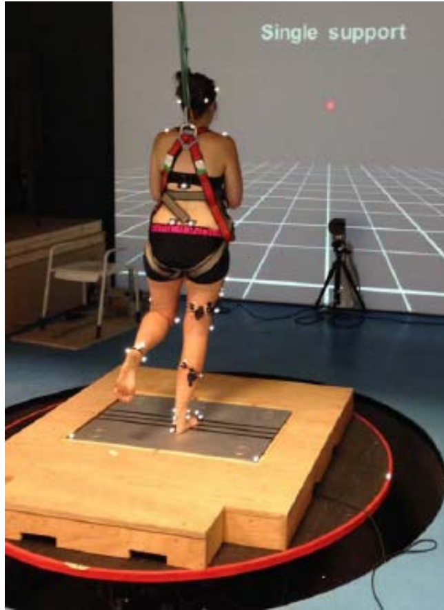
Figure 7. 1: CAREN System (MotekMedical), single-leg support setup.
