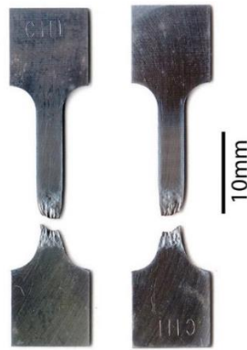
Figure 4.3 Fe-Cr-Al creep rupture specimen.
