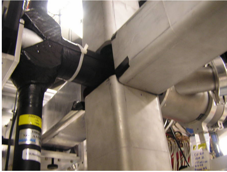
Figure 12: The four high purity germanium clovers and two plastic scintillators (covered in black tape) surrounding the site of implantation, which is inside the beam pipe.
