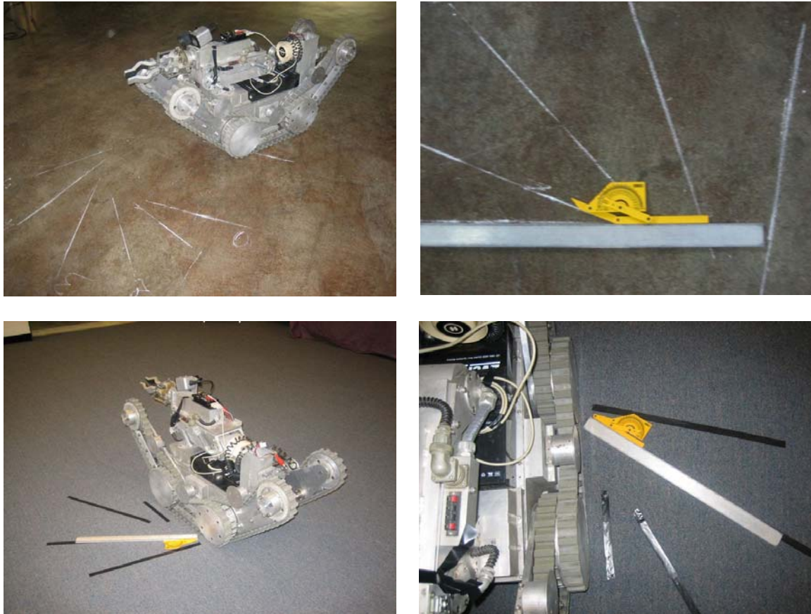
Figure 33: The pictures on the left show the methodology in measuring the covered angle for the same number of strings. The pictures on the right are close up images of the same process on both types of floors.
