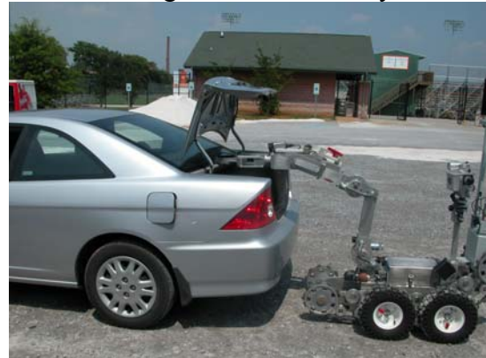
Trunk inspection by a robot.
