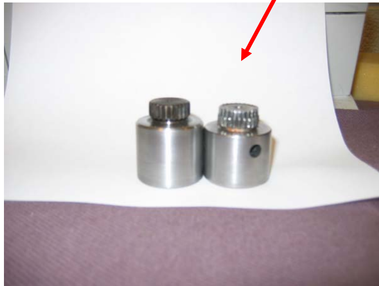
New Shaft and Original Shorter Shaft
