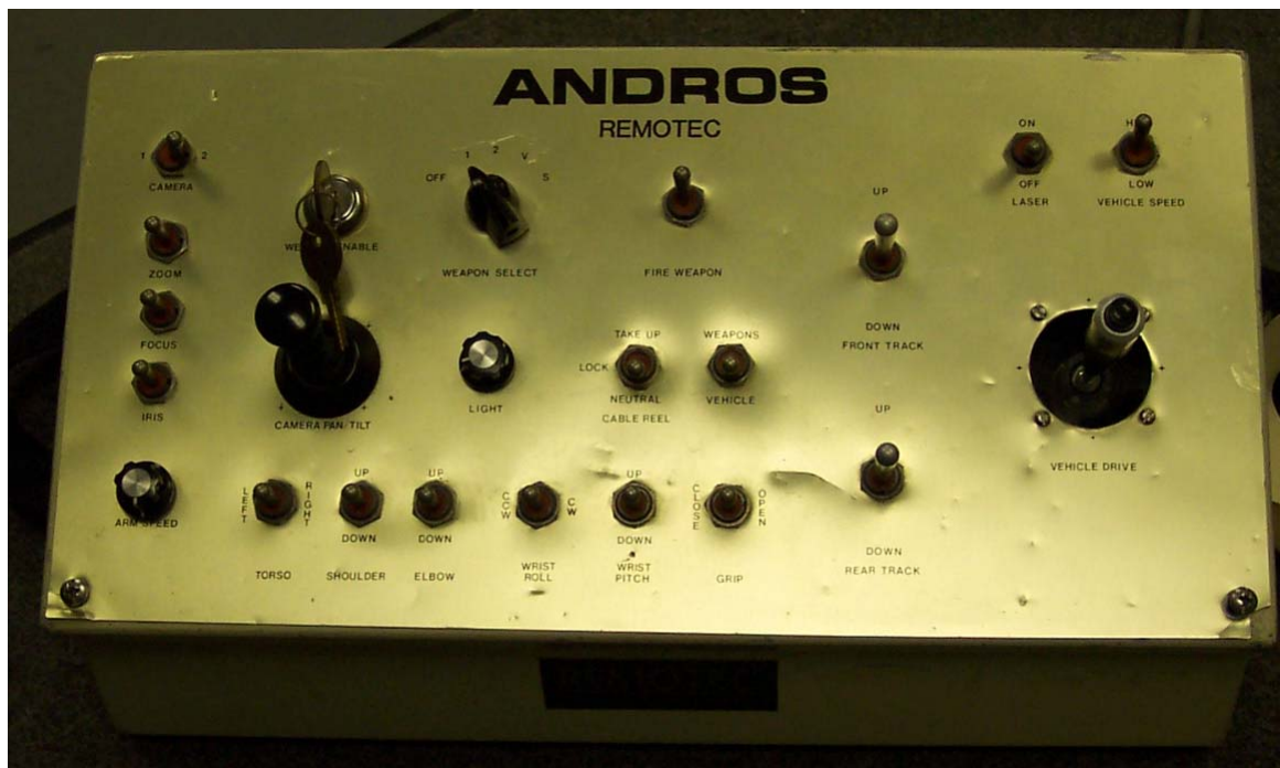
Figure 3: This figure show the original mechanical control panel for Remotec ANDROS Mark VA.
