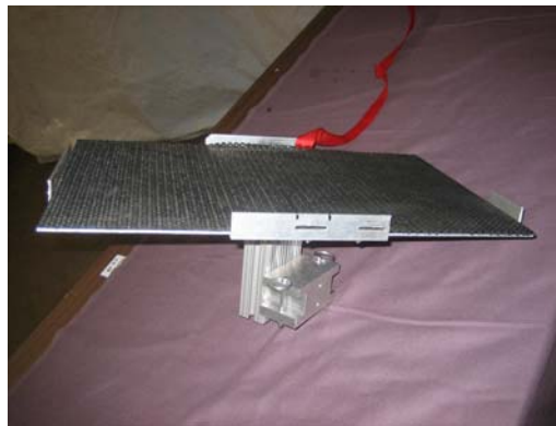
Figure 21: The brick carriage simply consists in an aluminum plate with constraints and an aluminum bar that links it to the robot. The red strap and the rubber film under the brick increase its stability.
