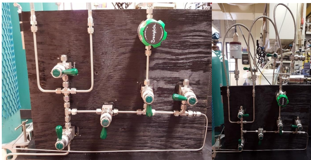
Figure 45. Photographs of the completed upstream assembly of the instrument.
