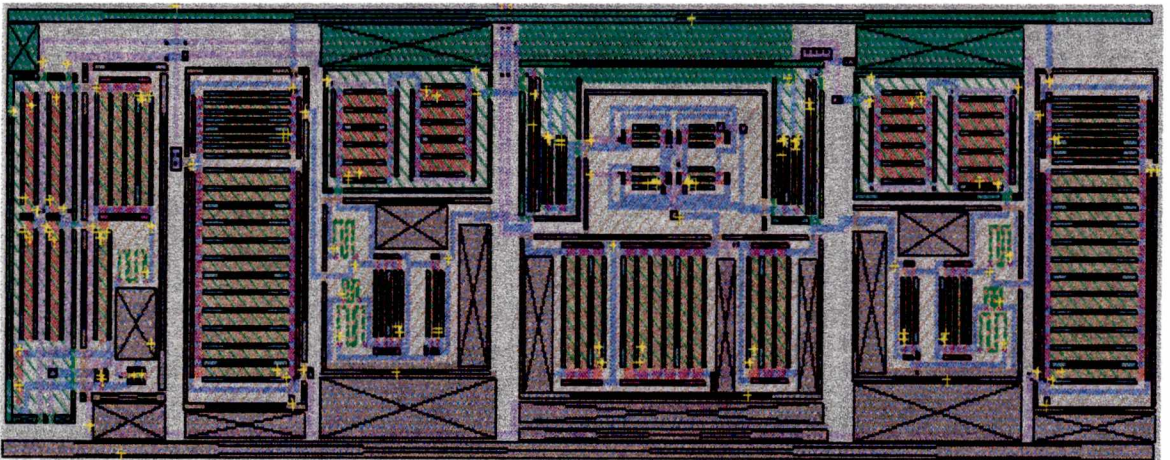
Figure 32 - MAGIC layout of transimpedance amplifier with current mirror stage for AMI 0.8 um run
