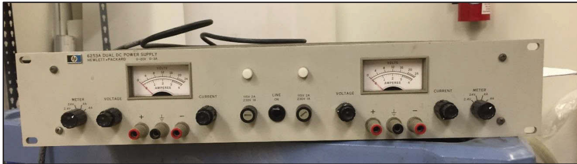
Figure 11. AC to DC power convertor (HP 6253A)
