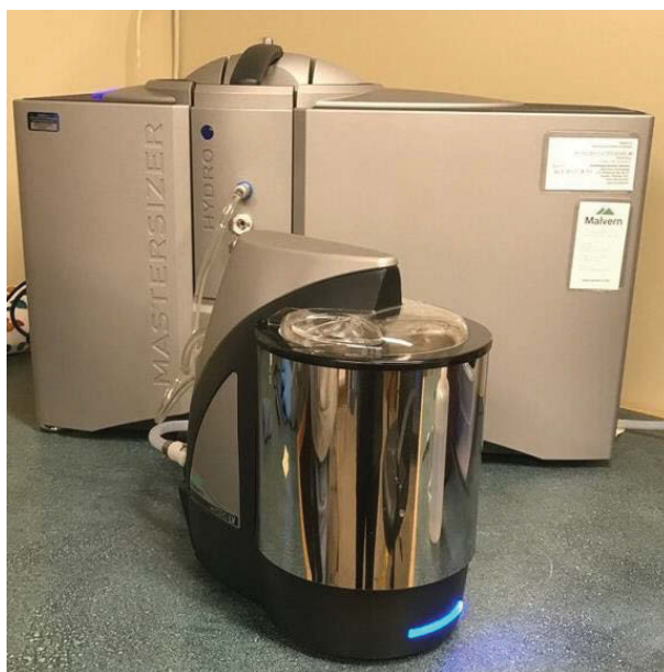
Figure 14. Visual representation of the Mastersizer 3000 and Hydro LV
