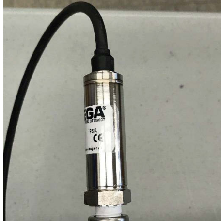
Figure 3. Visual representation of the absolute pressure transducer
