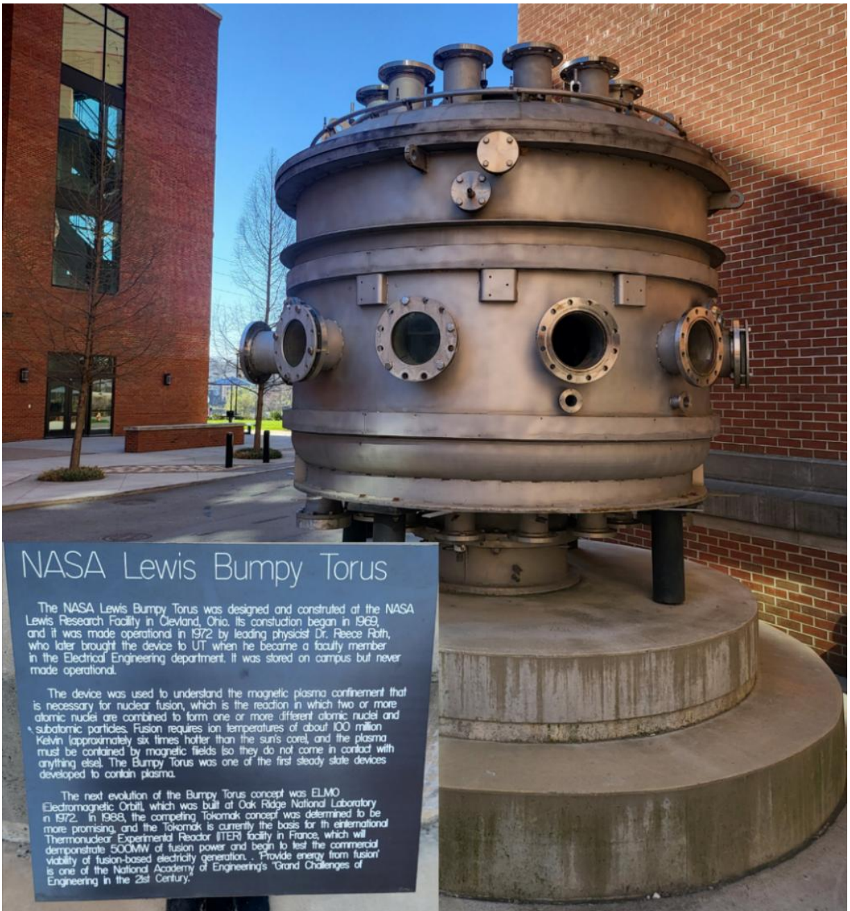
FIGURE 2. NASA'S LEWIS BUMPY TORUS USED TO TEST MAGNETIC PLASMA CONFINEMENT FOR FUSION SYSTEMS.
