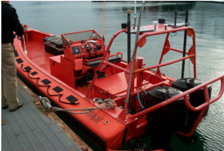
Figure 7. High Speed Maneuverable Seaborne Target (HSMST) 19
