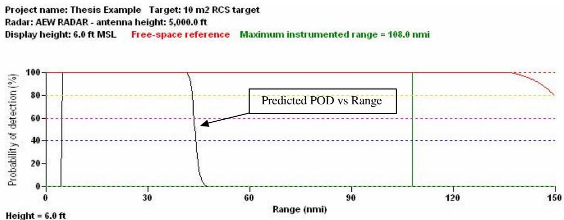
Figure 6. AREPS Probability of Detection (POD) versus Range<sup>16</sup>
