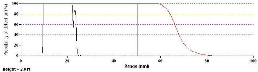
Figure 13. AN/APS-115 Short Pulse Mode versus 3m<sup>2</sup>RCS Target
