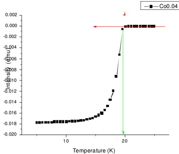
**Figure 22:** Method of  $T_c$  determination using tangent lines.
