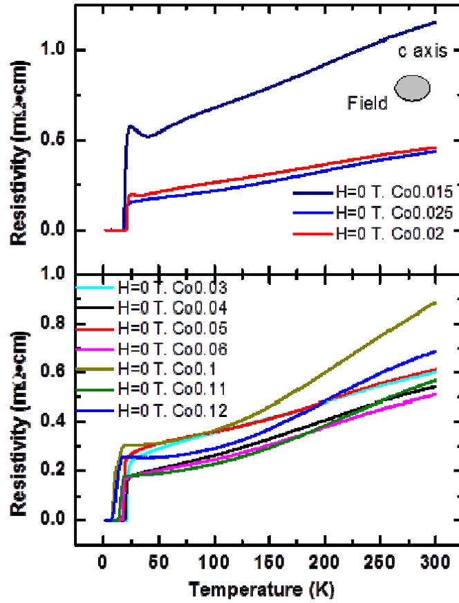
**Figure 21:** Resistivity measurements of compositions using a PPMS, courtesy of Dr. Guotai Tan.
