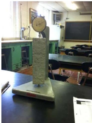
**Figure 8: Length Comparator for Shrinkage Testing**
