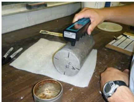
**Figure 3: Surface Resistivity (SR) Testing Apparatus**
