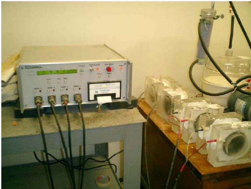
**Figure 1: Rapid Chloride Ion Penetration (RCP) Testing Apparatus**
