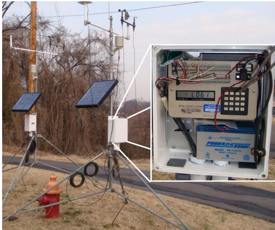
Figure 4. Typical weather stations and data logger used at study sites.
