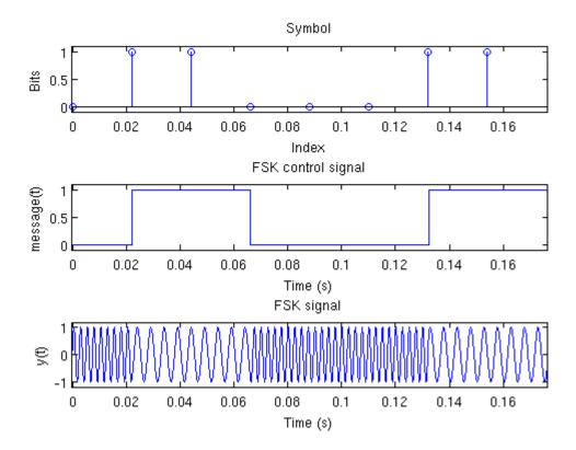
Figure 2: RTTY modulation example
