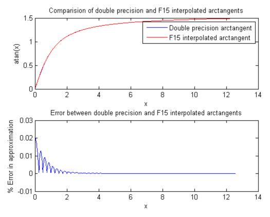
Figure 4: Comparison of double precision and F15 interpolated arctangents
