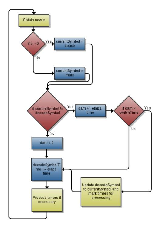
Figure 6: RTTY decode logic
