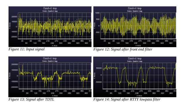
For the 3db signal to noise signal in the above graphs, the simulated RTTY demodulator produced the entire message "HELLO WORLD." For 0db, the simulated demodulator produced "HELO WORLD", and for -3db the simulated demodulator produced "HELO TRGL." As can be seen, as the noise becomes more prominent, the received message slowly degenerates to the point that it is uninterpretable.
