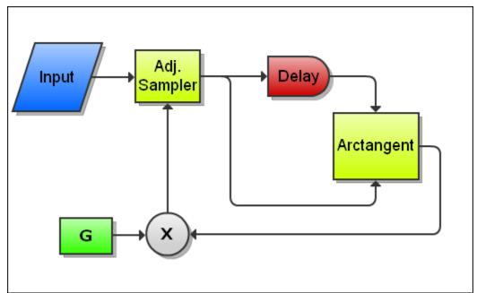
Figure 3: Time-delay tanlock loop diagram
