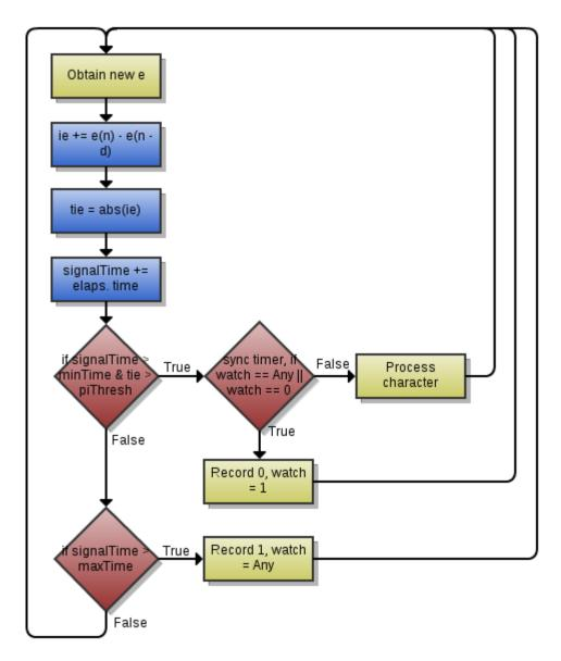
Figure 5: PSK31 decode logic
