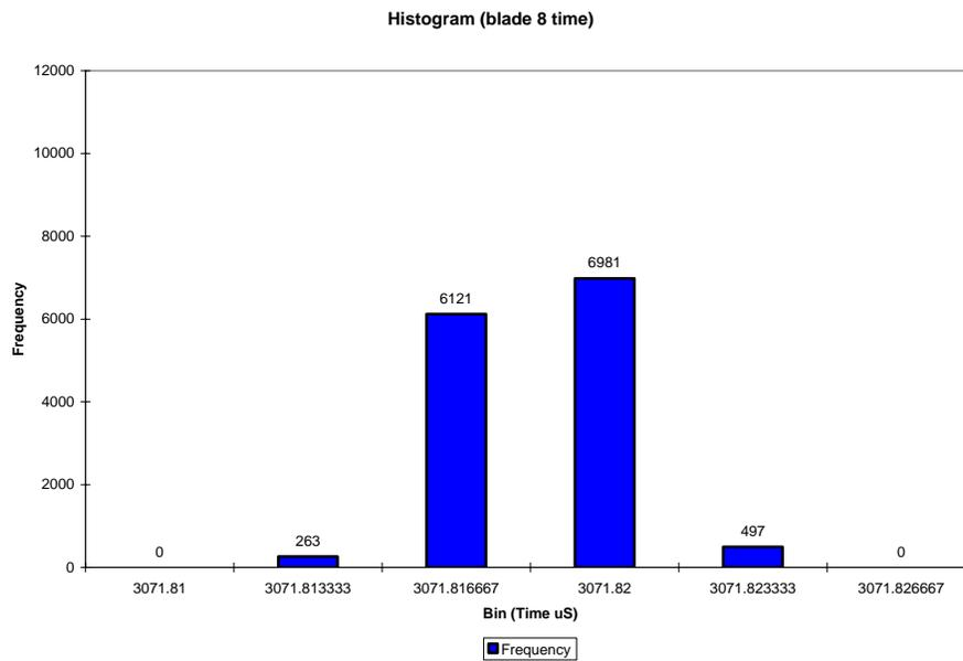
Figure 18. Histogram of Blade 8 time of arrival measurement
