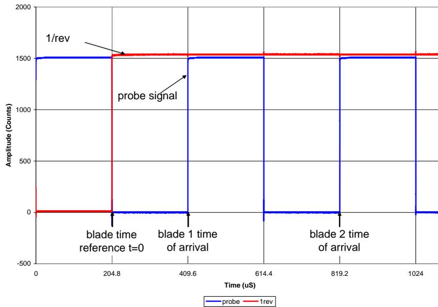
Figure 12. Stable input source probe and 1/rev signals
