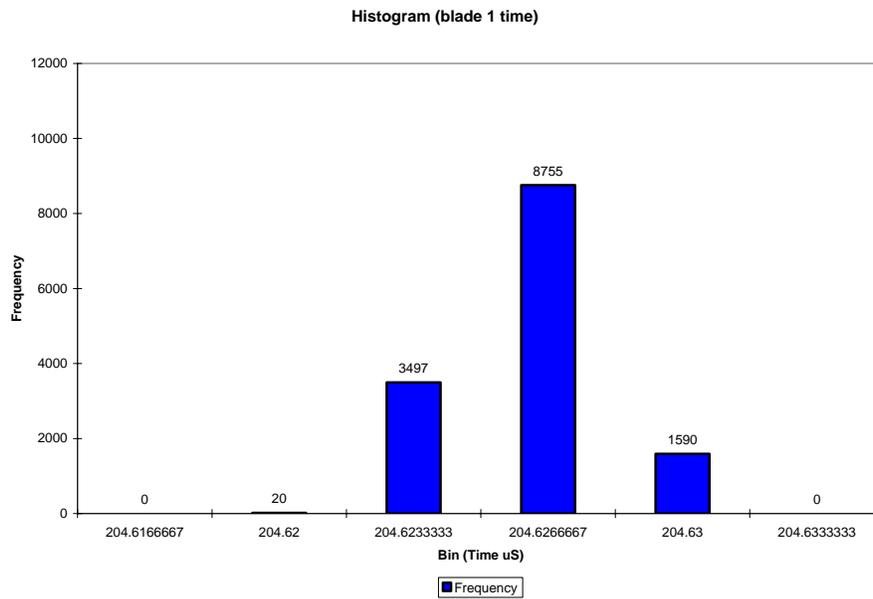
Figure 17. Histogram of Blade 1 time of arrival measurement
