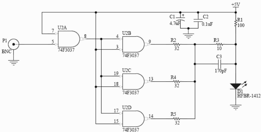
Figure 11. High speed fiber optic transmitter
