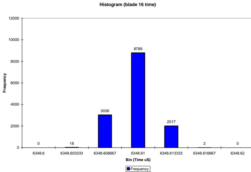
Figure 19. Histogram of Blade 16 time of arrival measurement
