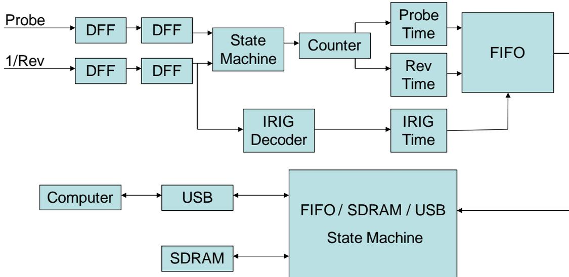
Figure 10. High speed counter design block diagram
