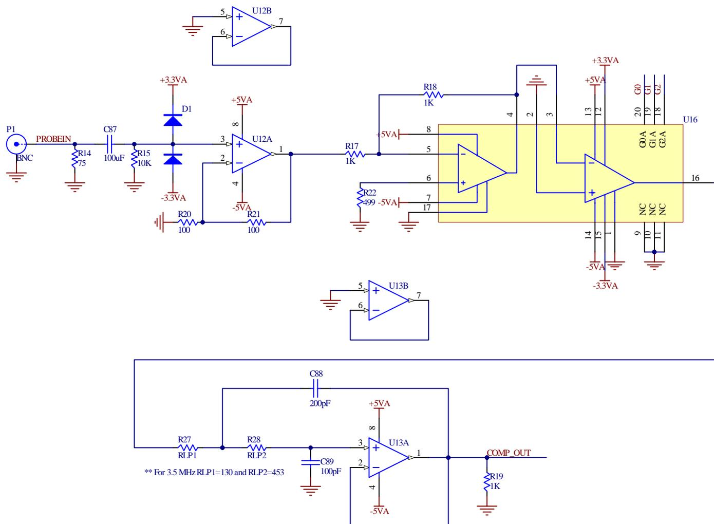
Figure 6. Analog signal conditioning schematic including variable gain amplifier and low-pass filter
