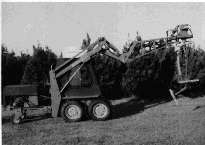
Figure 18: In the South, where topography is gentle and the summers are long and hot, shearing machines have been developed to shape Virginia pine. This species requires at least 2 shearings each summer. Photo credit: Murphy-Matic, Inc.
