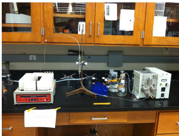
Fig. 2: This picture depicts the custom-designed soil column system used in this study. Depicted to the far right is the HPLC pump which actively pumped fluid through the Teflon and stainless steel tubing to the soil column. Fluid flowing out of the soil column was collected at regular intervals in quartz vials by a fraction collector system.
