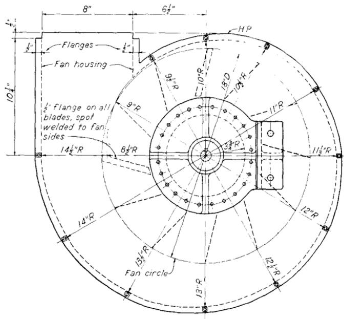
**FRONT ELEVATION-FAN HOUSING**
