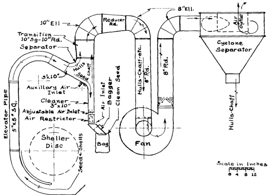
Fig. 5—Diagrammatic layout of elevator-separator-cleaner unit.
