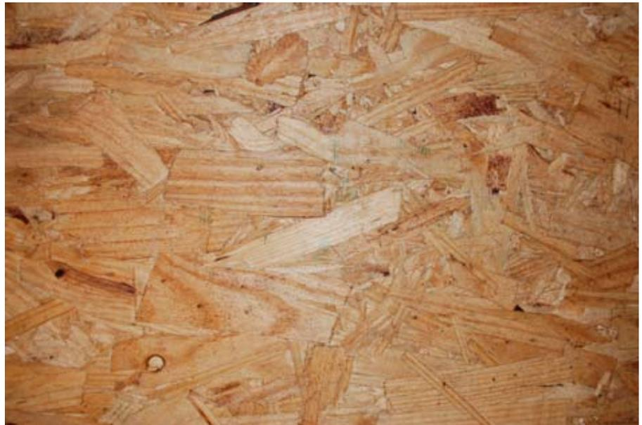
*Oriented strandboard (OSB) is made from thin flakes of wood that are glued together. OSB panels are commonly used as wall and roof sheathing and for subflooring.*
