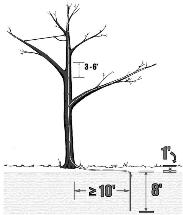
**Figure 1. A typical tree lightning-protection system. Fastener spacing is 3 to 6 feet. Ground rods (at least 8 feet long) should be driven in the ground at least 10 feet from the trunk. The top of the ground rod should be at least 1 foot deep.**
