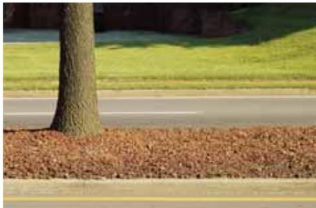
Crushed brick is an inorganic mulch that is decorative and long-lasting, being used on the median of a roadway.
