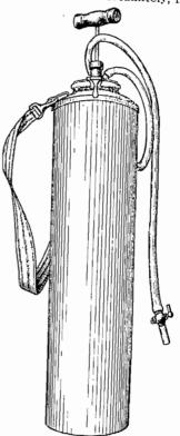
Fig. 2.—Compressed-air spray pump.
