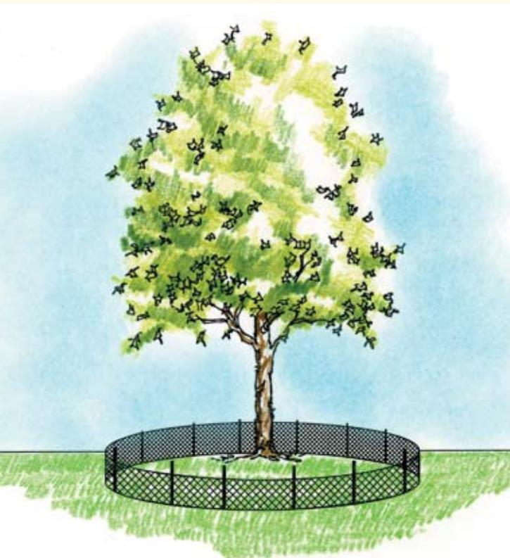
Figure 4. Protective silt fence located beyond tree's dripline.
