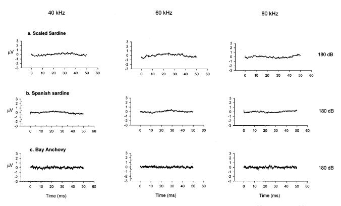
FIG. 3. ABR waveforms in response to 40, 60, and 80 kHz and at 180 dB for species that do not detect ultrasound: (a) scaled sardine, (b) Spanish sardine, and (c) bay anchovy. Arrows at 10 ms indicate troughs in ABR.
