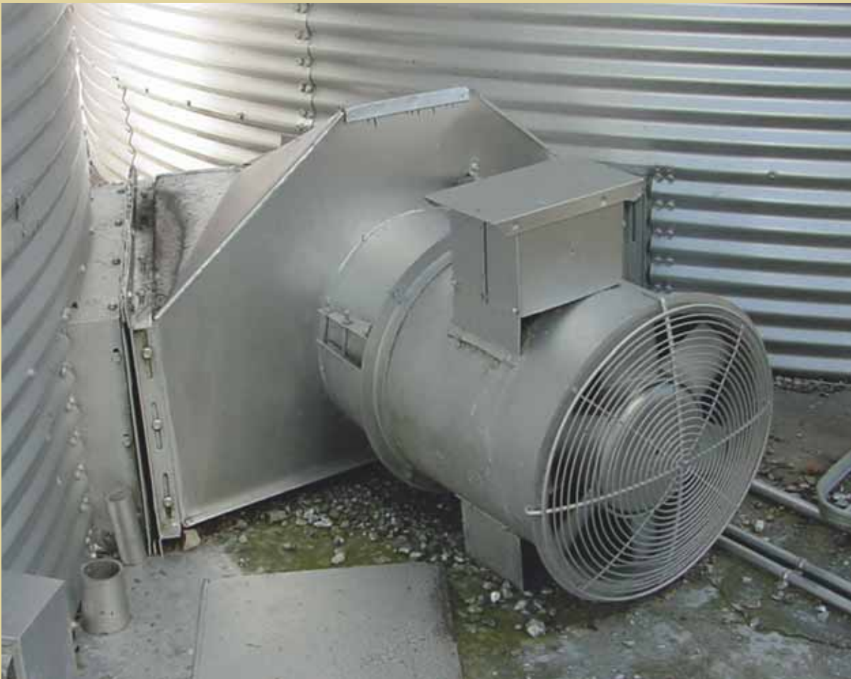
Aeration is a management tool that greatly improves the storability of grain.
