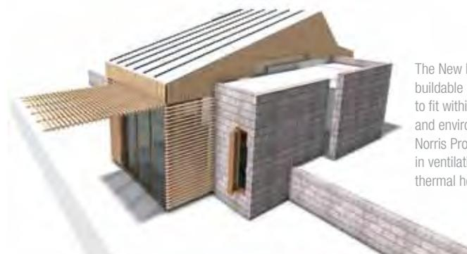
The New Norris House, designed to be buildable in the town of Norris, Tenn., and to fit within the architectural, technological, and environmental framework of the original Norris Project; it relies on advancements in ventilation, insulation, electric and solar thermal heating, plumbing, and lighting.
