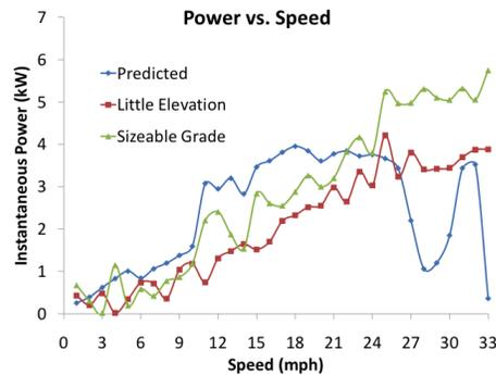
Figure 2. Comparing the instantaneous power vs. speed of the predicted needs, the little elevation route and the sizeable grade route.
