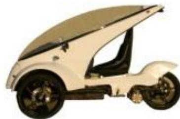
Figure 1. The commercially available BugE<sup>®</sup> frame and chassis kit.
