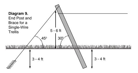
posts are suggested for Geneva double curtain trellises. The stability of an end post can be increased by setting or driving it so the aboveground part of the post is angled away from the vineyard at about 30 degrees from the vertical and braced or anchored (*Diagram 9*).
