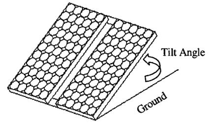
**Figure 4. Solar panel tilt angle.**
