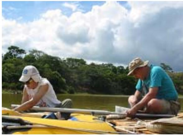
*Photo 3. Professor Sally Horn and Ph.D. student Marty Arford coring the sediments of a lake in northwestern Costa Rica. The core tube, full of sediment after a successful drive, is being removed from the drill string and sealed for return to the Paleoenvironmental Research Lab. A new, empty tube will then be attached so that the coring can continue.*
