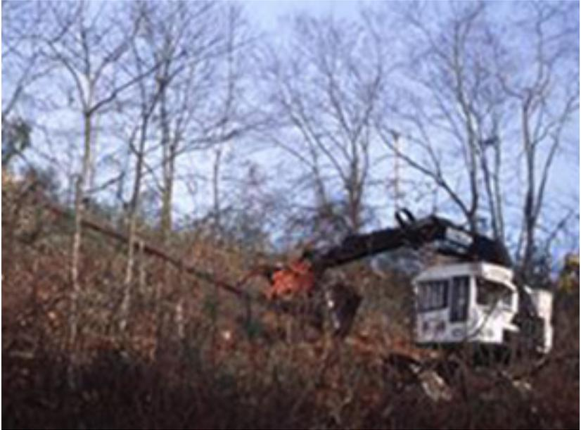
**Pines can be harvested using conventional chain saws, or with maneuverable fellerbunchers shown here.**
