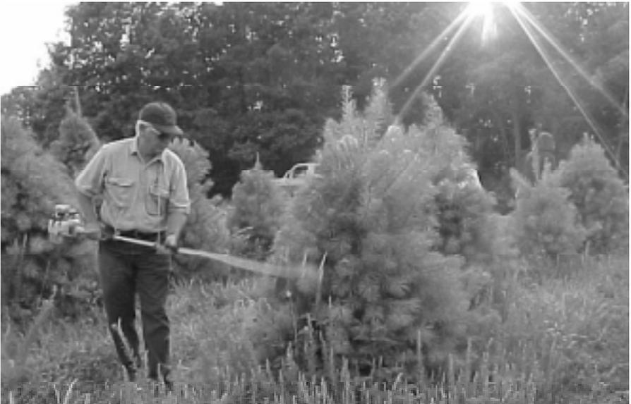
*Small gasoline-powered shearing machine.*
