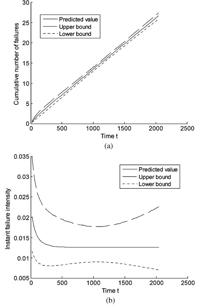
Fig. 5. Predicted (a) failure number, and (b) instantaneous failure intensity with 95% confidence bounds (2-sided)—new model with log-linear intensity.
