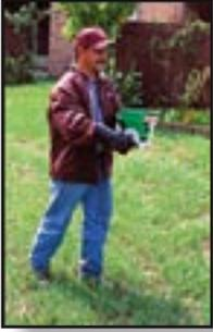
Hand-operated spreaders such as the EarthWay® Ev-N-Spred and Scott's® HandyGreen® are ideal for treating small areas with fire ant baits. The operator can walk or ride on the back of a vehicle. Some push-type applicators, such as Spyker® Models 24 and 44, also may be suitable, but some modification (attach
